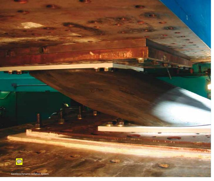
24 natural rubber isolators (16 lead core) will be used for the base isolation system. In the image, an example of one of those devices. Courtesy of RBA and DIS.
