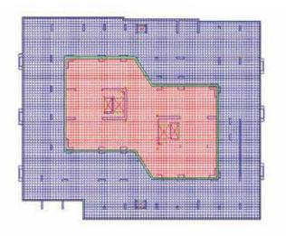
Project Outline: Blue represents the not isolated area corresponding to near 3.700 m2 of underground, while red refers to the isolated area of 1.400 m2 (base plate where the devices will be placed). Green refers to the 50 cm expansion left to avoid collision between the two buildings. Courtesy of René Lagos Engineers.
